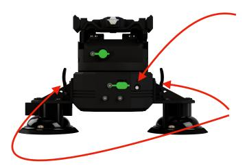
Press On/Off Button for 2 Sec. to switch on or off XR-II XR-II starts blinking and starts calibration Mode XR-II stops moving when calibration Mode is done Fast Blinking = XR-II is not balanced (open clamping levers and bring XR-II in balance)
