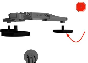
Clean the magnet foots and the to mounting surface carefully
