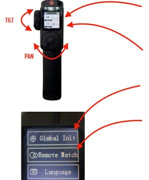
Press On/Off Button for 2 Sec. to switch on or off Remote Control Now your XCROW is ready to use.
